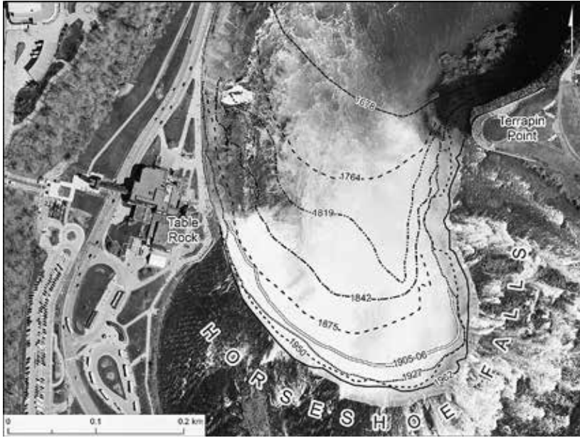
FIGURE 0.4 Historical erosion at the Horseshoe Falls (lines indicate crestline at a given year; aerial image is from 2017). Map by Jason Glatz (Western Michigan University Libraries) and Daniel Macfarlane
